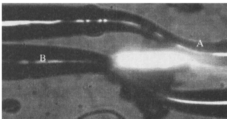
PICTURE 4 Coupling of light between two strongly bent fibers via index oil.
